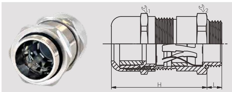
In the case of the **Euro-Top EMC Ampacity**, two EMC contact spring systems were compared, which leads to an increase in the contact cross-section between the cable shield and the cable gland. This significantly increases the current carrying capacity of the gland, which is beneficial, among other things, for rail applications.
